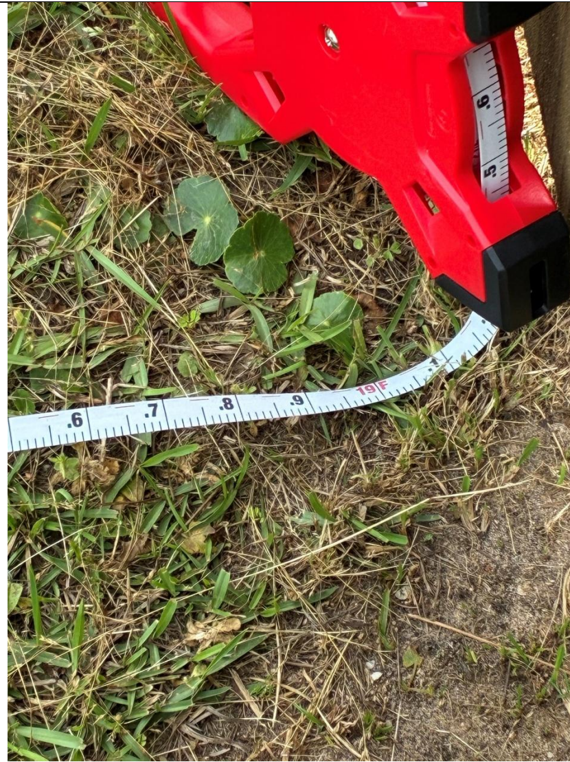
Photos 1 and 2: Measurement of distance from silt fence to western edge of Madison Place | 25 ft. ingress and egress and drainage easement is approximately 19 ft. This distance including appropriate buffering should exceed 25 ft.
